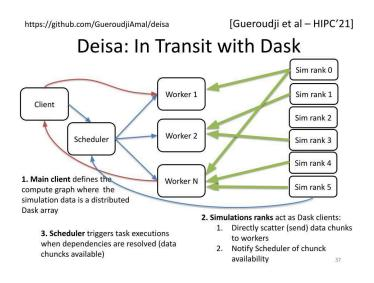
Compared to previous in situ approaches that are mainly MPI-based, our approach relying on Python tasks makes for a good tradeoff between programming ease and runtime performance.
